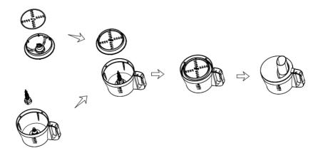
Note: Please refer to above FIG for installation, always place the driving shaft first then place the disc and disc holder combination together before placing into the bowl.
